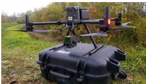
Figure 1. DJI Matrice 300 and DJI Zenmuse P1 camera.
