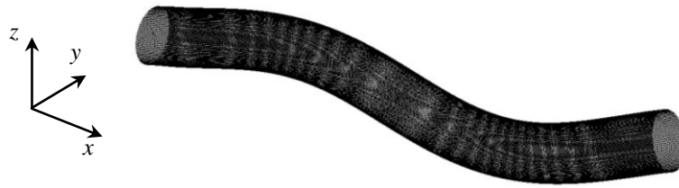
Figure 12: 3 rd flexural mode (3F, f = 1,835 Hz).
