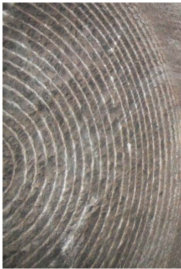
Figure 3: Chip formation due to TBM disc motion: scheme of rock destruction mechanism under a disc.
