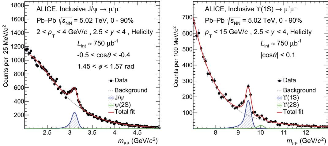
**Fig. 1.** Examples of fits to the invariant-mass distributions in the helicity reference frame. The left plot corresponds to the  $J/\psi$  mass region, while on the right a fit to the  $\Upsilon(1S)$  mass region is shown. The fits are performed using an extended Crystal Ball function for the resonance signals, while the background is parameterized with a variable width Gaussian.
