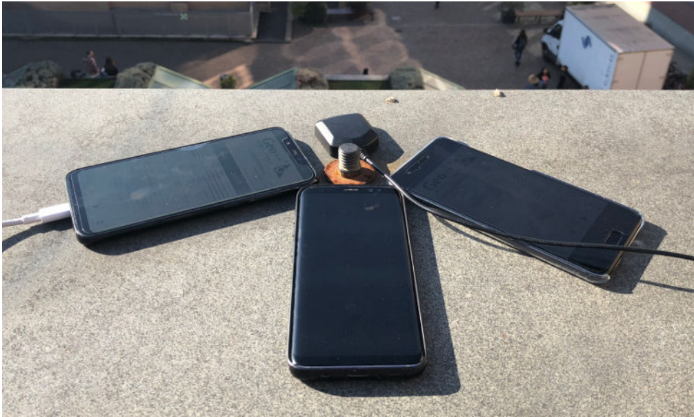
Figure 4.1: Set-up of the data campaign carried out using smartphones. The screw indicates the geo-referenced known point.
