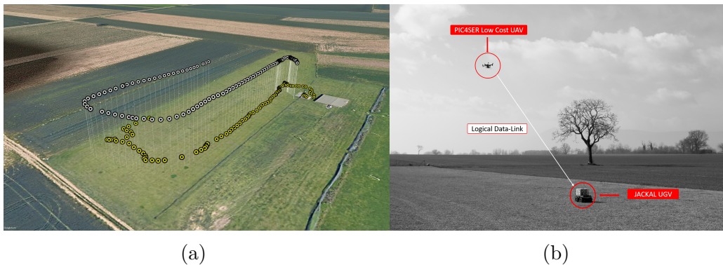
Figure 5.9: GNSS fixes of UAV and UGV in follow-me configuration shown in Google Earth (5.9a) and in real scenario (5.9b).
