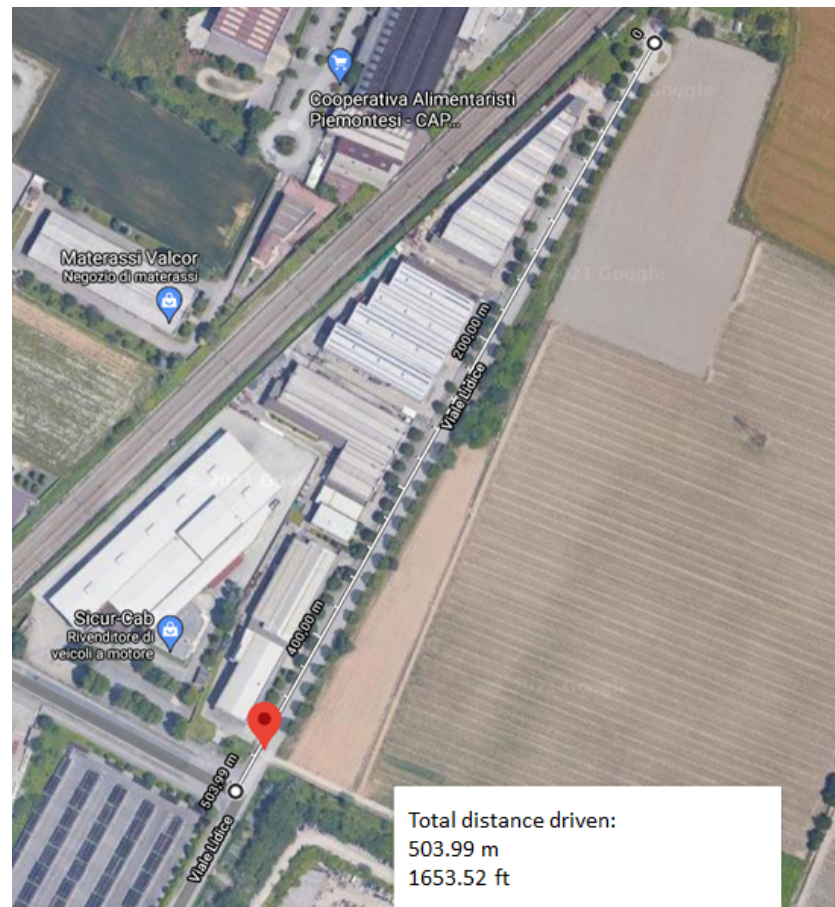
Figure 8. Selected route in Turin, Italy, for performing on-road tests for the prototype two-wheeler. The route is driven to calibrate the dynamic vehicle model.
