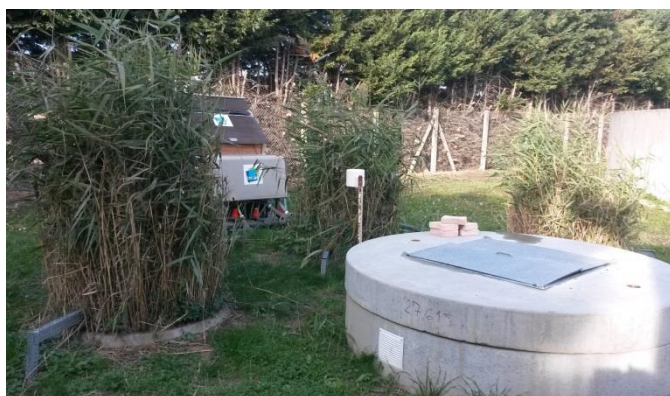
Figure 6: The three lysimeters containing the three soils studied (left); Phosphate fluxes measured at the inlet and outlet of the three lysimeters (right)
