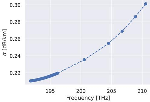
Fig. 2. Characterization results: loss coefficient function,  $\alpha(f)$ .
