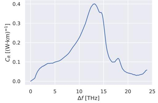
Fig. 3. Characterization results: Raman efficiency  $C_R(\Delta f)$ .
