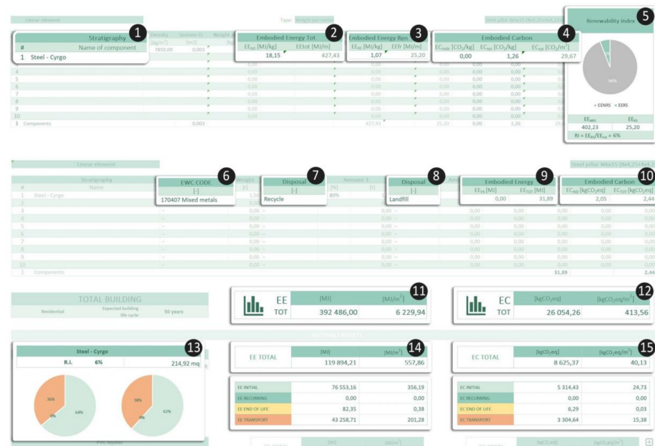
Figure 3. The figure shows the EURECA main results: numbers 1 to 5 refer to EE, EC, and RI of the material, or the building system; numbers 6 to 10 refer to EE and EC of the materials matched to the EU waste code; numbers 11 to 15 refer to EE, EC calculated for the building as a whole.
