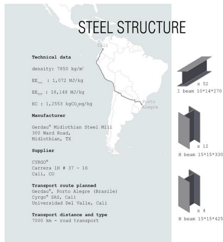
Figure 6. Data collection sheet for materials used in the PEI Maquina Verde’s House. The example refers to the steel structure. In the sheet are reported the main material features ( technical data ), information about the production site ( manufacturer ) and the distribution site ( supplier ), route, distance, and type of transport from manufacturer to supplier(s), from the supplier(s) to construction site ( transport planned route and transport distance and type ). (Source: Federica Gallina, Benedetta Quaglio).
