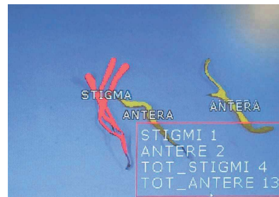
Fig. 7. Image of the PC screen with the computer vision output
