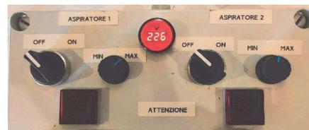
**Fig. 5.** The control panel with the voltmeter of the mains voltage, two rotary switches to turn on/off the aspirators, the potentiometers to set the speed, and two voltmeters/ammeters indicating the voltage and current supplied to the aspirators.
