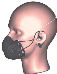
Fig. 4 The lateral perspective in the dummy head wearing the AG-47 SmartMask shows both the intraural thermal sensor and the pulse oximetry sensor at the ear lobe
