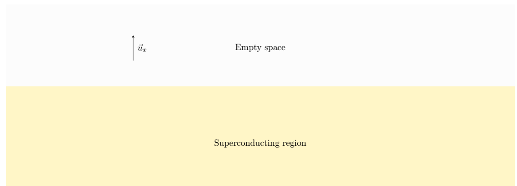
Figure 8. Half-infinite superconductor approximation. The Earth's gravitational field is parallel to the \vec{u}_x direction.
