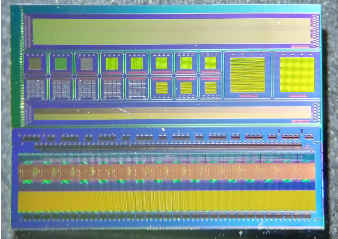
Figure 2.14: Microphotograph some of the new test structures included in the first engineering run of the ARCADIA collaboration. The long test structures are passive microstrips with different pitches, while the square ones are mostly pseudo matrices with different pixel geometries. At the bottom an active pixel array has been included to test new readout architectures.
