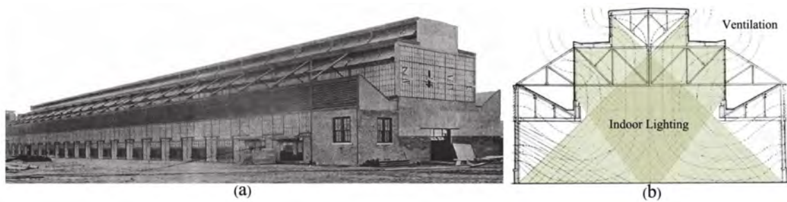
Figure 9. The forging workshop of the Packard Plant: (a) the facade and (b) the section. (Source: [8]).
