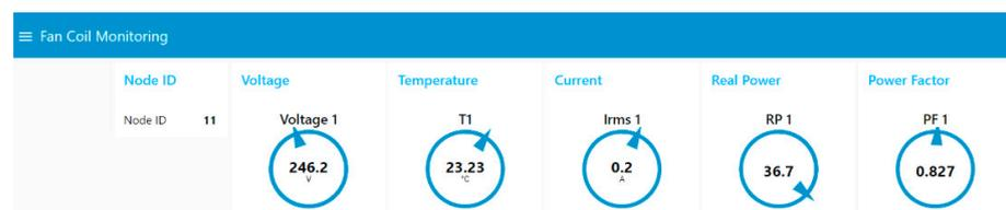
**Figure 12.** Node-red monitoring dashboard in real time.
