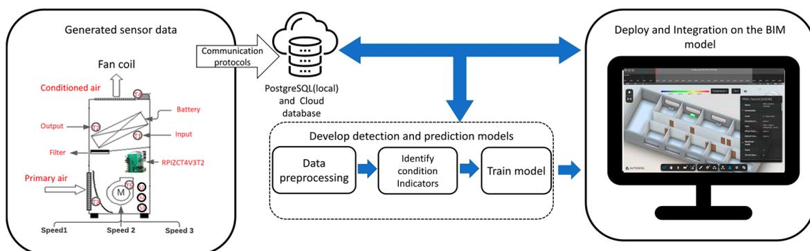
**Figure 1.** ML-based building facility anomaly prediction framework.
