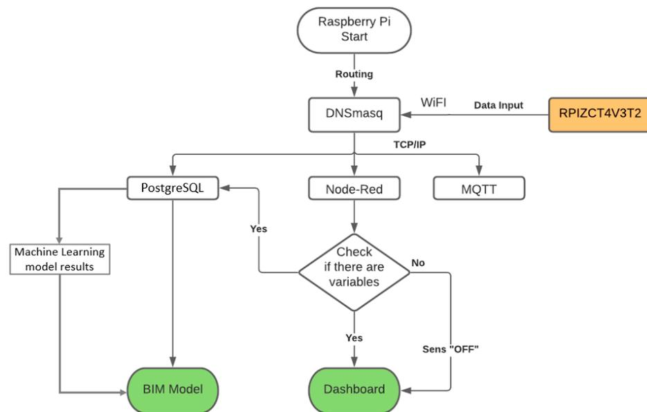
**Figure 3.** Functional flowchart of the framework.
