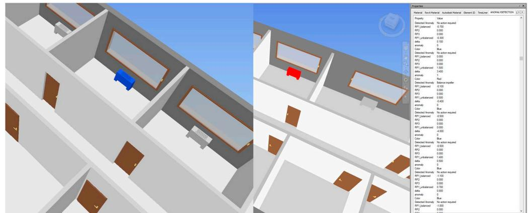
**Figure 11.** Autodesk Navisworks custom 3D BIM model integrated with IoT and ML results data: on the left, balanced condition is colored with a “Blue” and on the right, the motor is under unbalanced condition and colored with a “Red”. Turned off FCs are colored with a “Grey” color.
