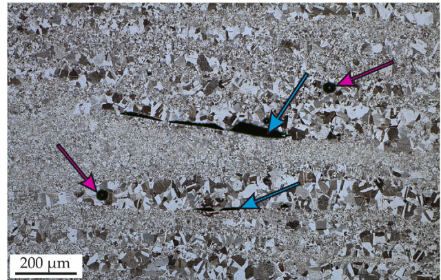
Figure 4. Visible light microscopy image of the occurring porosities in EBM Ti-48Al-2Cr-2Nb. Whereas spherical pores stem from Ar-entrapment (magenta arrows), elongated pores between adjacent powder layers form due to unfavorable process parameters (blue arrows). This lack of fusion porosity exclusively appears below the large \gamma -grain bands, which, therefore, represents the non-Al-depleted zones toward the bottom of melt baths. The building direction is upwards.
