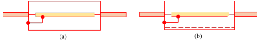
Fig. 5. Metal box screening a grounded circuit: (a) initial design; (b) improved design with insertion of a HIS.
