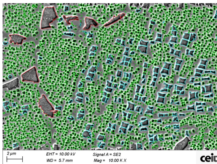
Figure 4. FEG-SEM image of a typical standard HTed Astroloy microstructure taken with the secondary electron detector. \gamma' are coloured with red for primary \gamma' , blue for secondary \gamma' and green for tertiary \gamma' .
