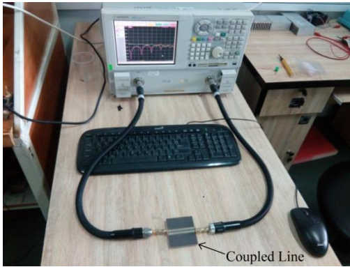
Figure 6: The experimental setup of measurement of a microstrip coupled line.
