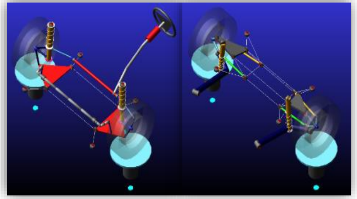
FIGURE 2 Front (MacPherson) and rear (multilink) suspension
