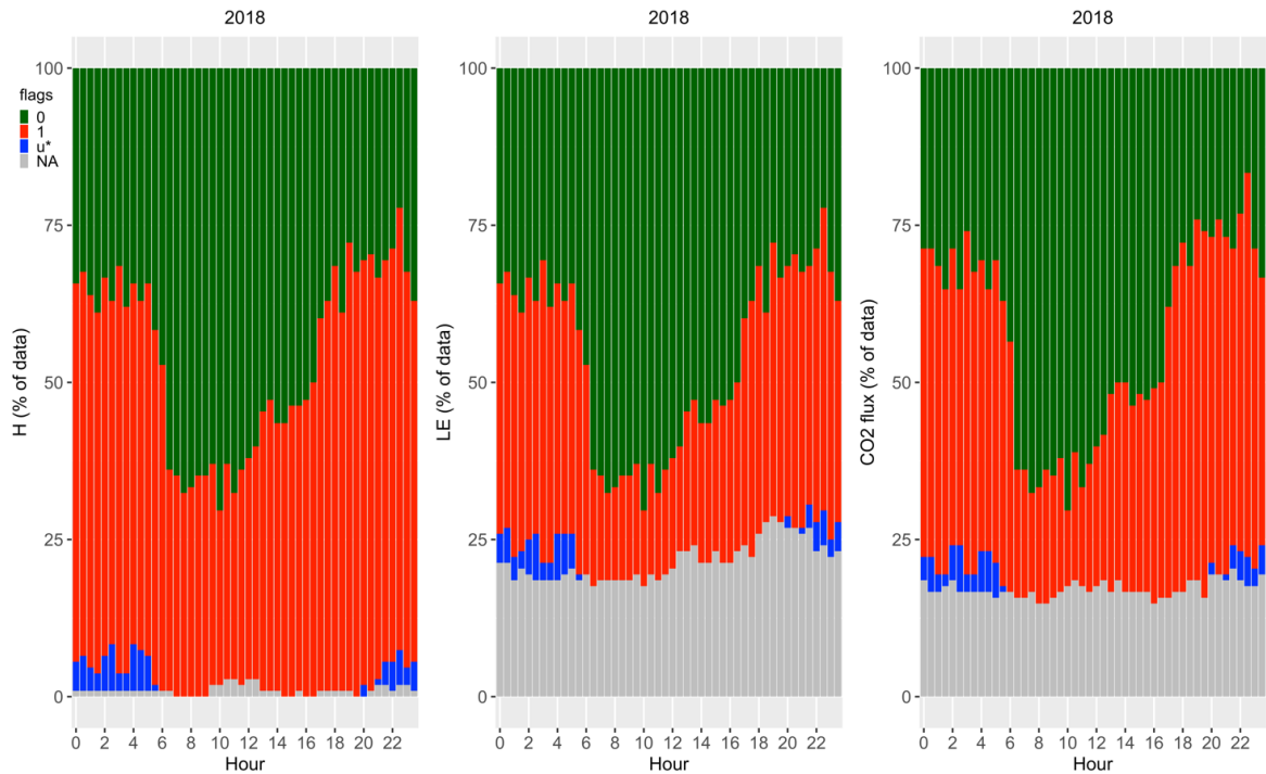
Figure 4.20. Overall flag, missing data and friction velocity flag. Green: data passing the overall flagging system without test on low friction velocity; red: bad quality data; blue: data passing the overall flag but not the friction velocity test. Grey: missing data.
