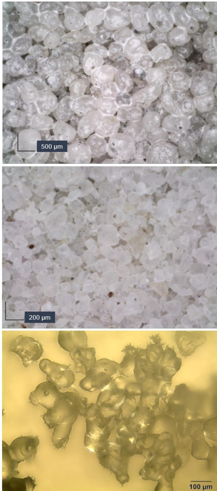
**Figure 3.3** *Enceladus simulants. Fine-grained pervious concrete (Top). Very fine-grained pervious concrete (Middle). Sintered cryogenic ice (Bottom).*
