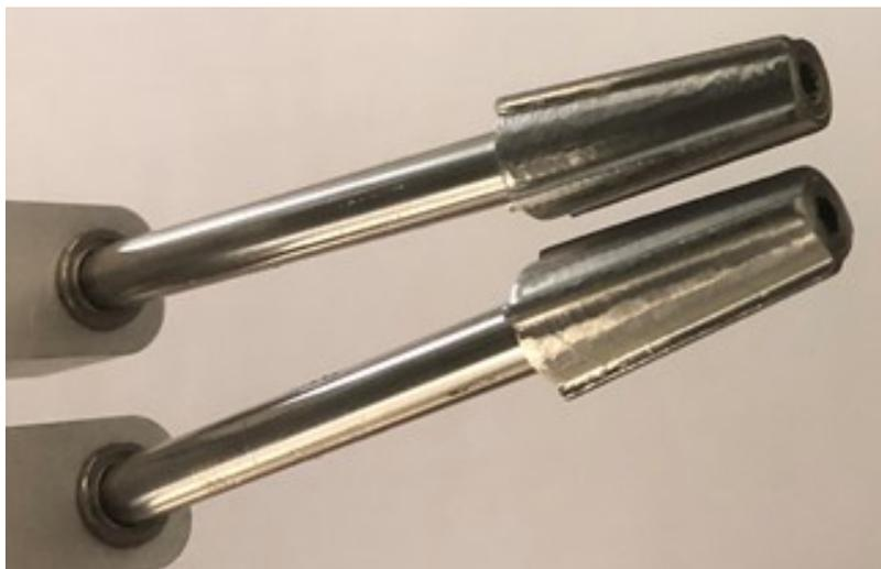
*Figure 3.22 Dual-Rasp cutters. The two counter-rotating, rasp-type cutting heads remove the pristine material and throw it up between them via momentum transfer.*
