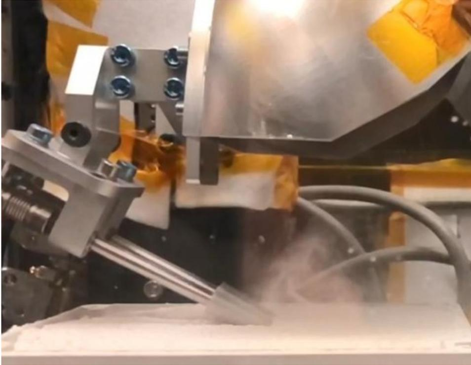
*Figure 4.61* Sample transport of approximately  $10\ \mu\text{m}$  particles in 1 atm conditions.
