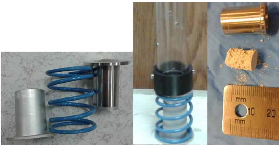
**Figure 3.11** Implemented drive tube components (Left), assembled (Middle), and sample tube with collected sample (Right).
