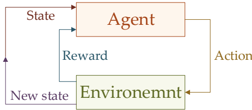
Figure 2. Block diagram of reinforcement learning (RL) control.
