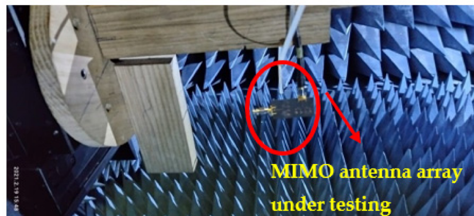
Figure 6. Proposed MIMO antenna array under testing.
