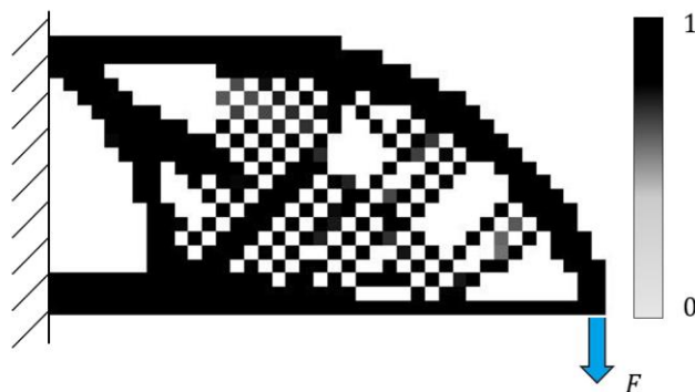
Figure 22 - Checkerboard effect on final topology
