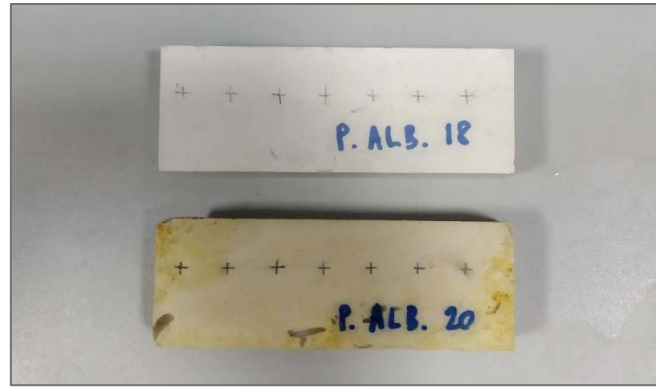
Figure 13: Visible staining as effect of temperature and moisture on the he specimen P ALB 20 in comparison with P ALB 18 in natural conditions.
