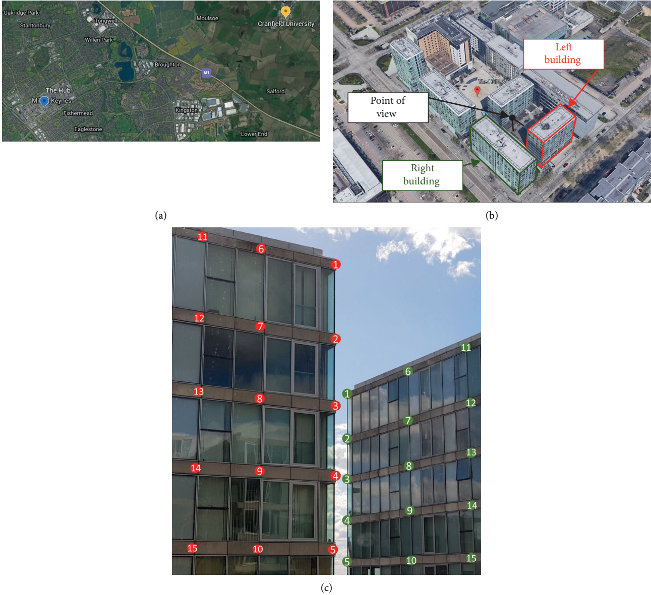
FIGURE 11: (a) Location of the in situ survey. (b) Satellite view of the surveyed area. (c) The first frame of the recorded video, with the position of the 30 virtual sensors highlighted.
