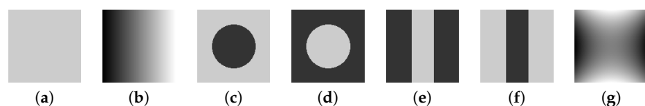
Figure 12. The seven archetypal image patches of the BIF: flat area (a), gradient (b), dark spot (c), bright spot (d), bright edge (e), dark edge (f) and saddle (g).
