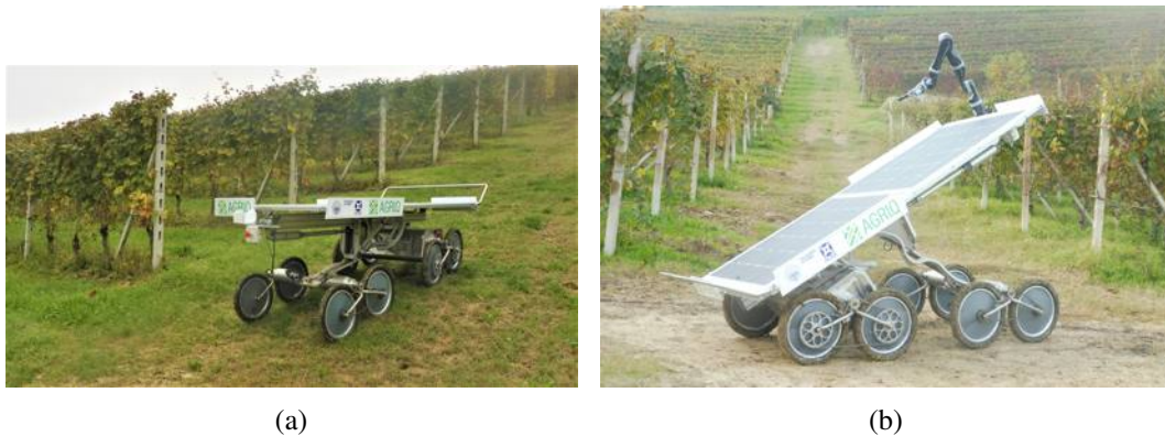
Fig. 2.20 (a) Agri.Q panels compensating the hill incline. (b) Agri.Q at its maximum pitch angle
