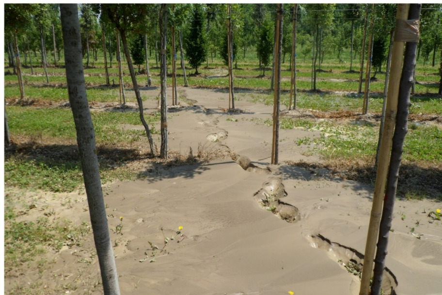
Figure 3. (a) Location of the boreholes sampled for classification tests; (b) Uccivello sand boil.
