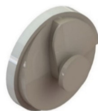
Figure 9. Three-dimensional (3D) computer-aided design (CAD) model of the proposed cam.
