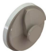
Figure 9. Three-dimensional (3D) computer-aided design (CAD) model of the proposed cam.
