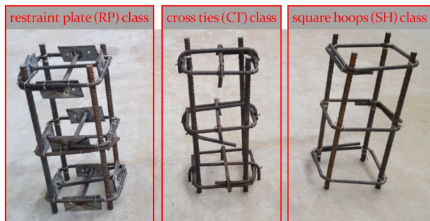
Figure 2: Different arrangements of transverse reinforcement considered in this experimental campaign: RP class (left), CT class (center), SH class (right)
