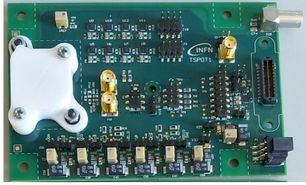
(b) TSPOT1 PCB. Board size: 8 cm \times 12 cm. The ASIC is mounted on the left side under the white removable cover.
