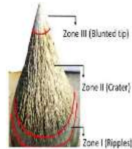
Figure 3. Blunt needle tip subjected to high pressure (Din and Harmain 2020)
