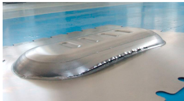
Fig. 4 Photograph of the deformed Ti6Al4V sheet
