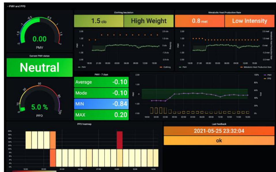
Figure 9. Sample view of the first dashboard section: PMV and PPD.
