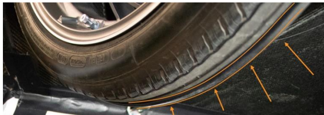
Figure 3 Rubber circumferences around JUNO's tyres
