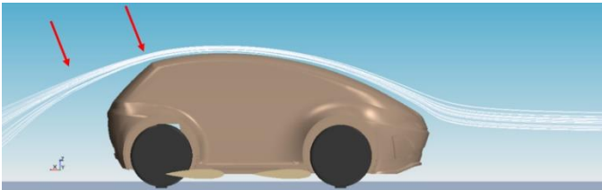
Figure 32 Standard configuration, JUNO's CFD streamlines scene
