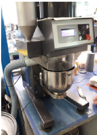
Fig. 2. From left to right Hobart mixer assembled, B-flat beater and mix device bowl with the soil and foam before mixing (Unit: mm).
