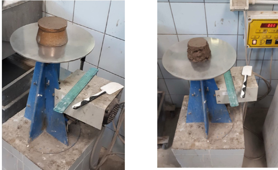
Fig. 3. The mini cone on the flow table filled with soil and after the lifting of the mini-slump cone. The dimensions of the used mini-slump cone are: Height is 60 mm; Diameter of the upper face is 70 mm; Diameter of the lower face is 100 mm.
