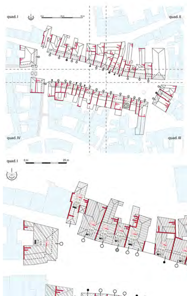
Figure 7. Overview relative to the case study of Piazza di Santarosa – Savigliano: resistant system, geometric conformation and conditions relating to the single building and interaction between adjacent buildings forming a standardised aggregate (ref. Tab. 1 – 15). (edited by Vincenzo Donato). Enlargement of quadrant I: case study of Piazza di Santarosa (ref. Figure 7) - (edited by Vincenzo Donato)
