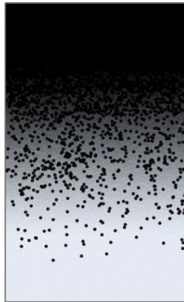
Fig. 1.5: Composition of materials in microstructure of FGMs
