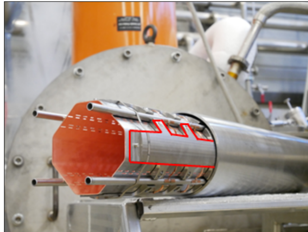
Fig. 8.7 A photograph of a beam screen for HL-LHC (© 2018 CERN). The tungsten insert is highlighted in red.
