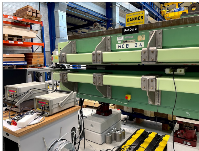
Fig. 6.11 A photograph of the dipole magnet used as a field source.
