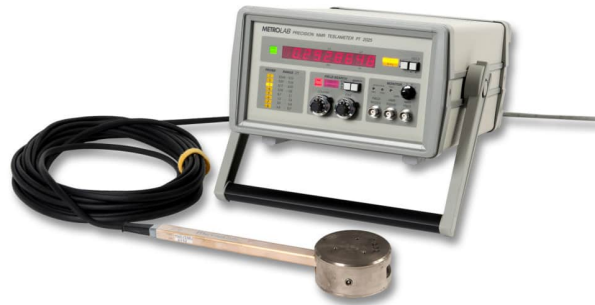
Fig. 6.9 A photograph of the NMR Metrolab Pt2025 from [189].
