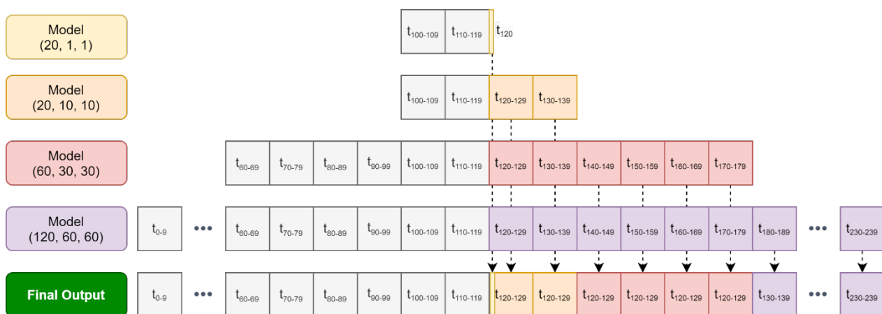
Figure 7. Process of stacking different results coming from different neural networks. Grey squares represent inputs, while yellow, orange, red, and purple squares denote outputs for each model denoted by corresponding triplet (I, O, F) . Last line outlines final output, concatenation of all different contributes.
