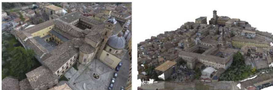
Plate 1. Image acquired by UAV during the data acquisition and the point cloud obtained
