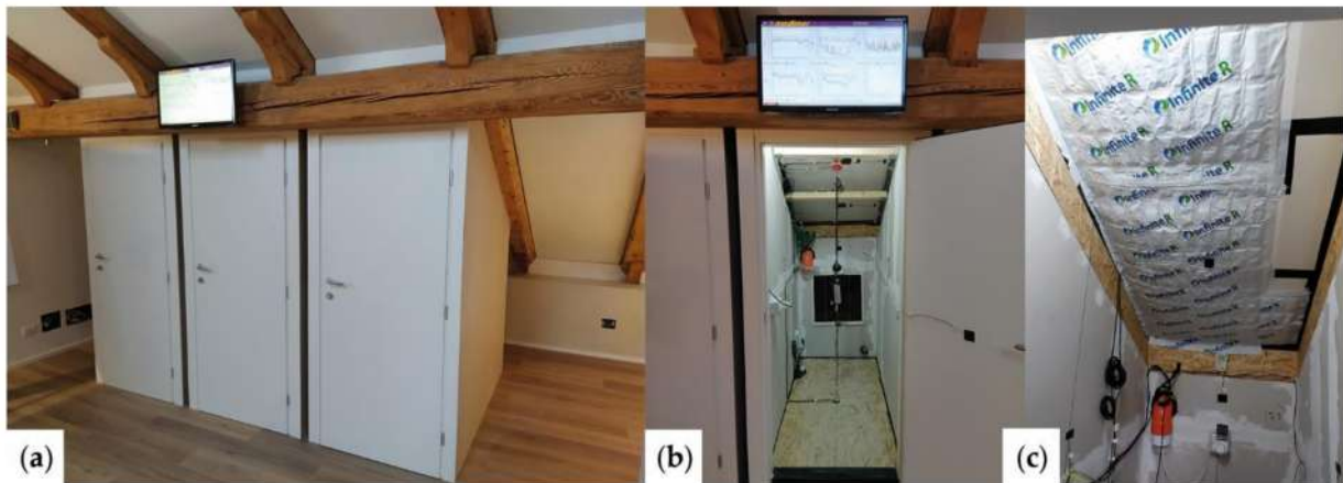
Figure 2. (a) The TRIS apparatus; (b) View of the internal space of a cell; (c) Installation of the Infinite R TM panels.
