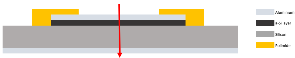
Figure 5. 7. Cross section scheme of device adopted for a-Si layer resistance evaluation. Measures are performed perpendicular to wafer (red arrow).
