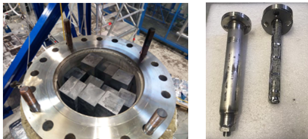
Figure 6: Melting furnace charged with LiPb ingots on the left and LiPb filter installed between melting tank and storage tank.
