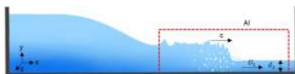
Figure 1. Illustration of the positive surge wave, where AI indicates local refinement zone. Surge Froude number is Fr = \frac{c + U_1}{\sqrt{gd_1}} , where U_1 is the velocity downstream of the wave and c is the celerity.
