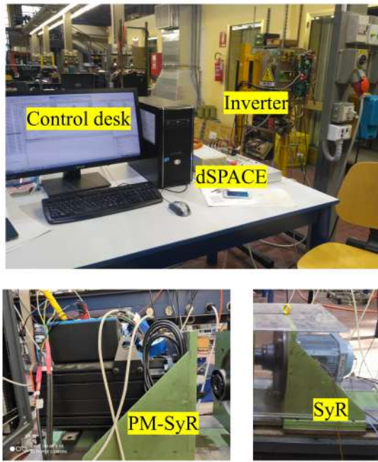
Fig. 9. Experimental Setup of 1.1 kW SyR and 11 kW PM-SyR motors under test on a dSPACE DS1103 control platform.
