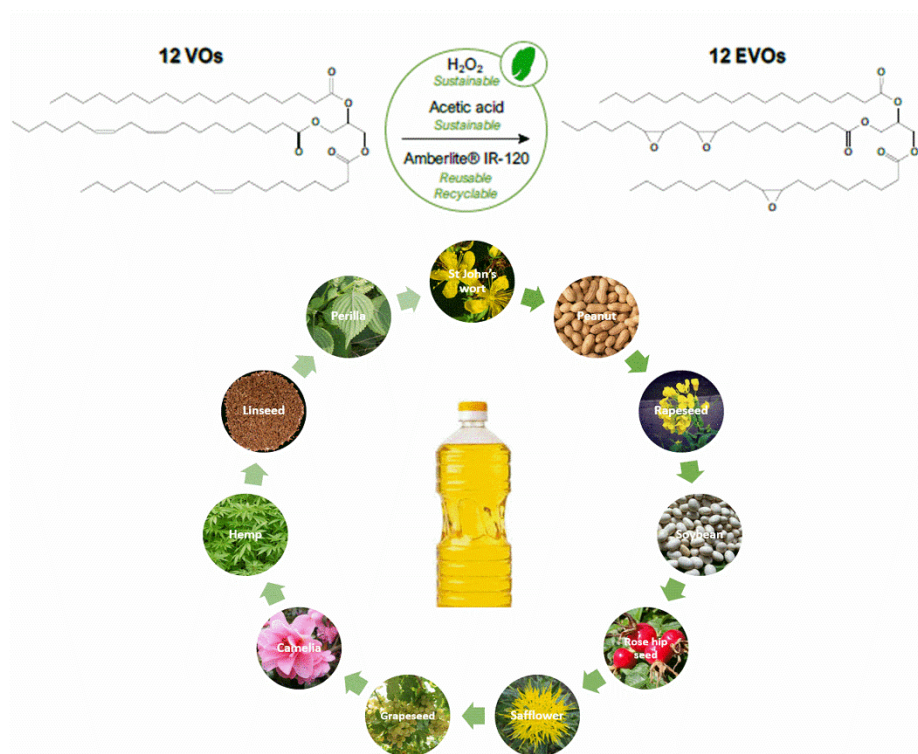
Figure 3.8: List of the twelve vegetable oils epoxidized with a green synthesis procedure by Specific Polymers used in this work.
