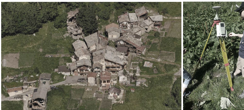
Figure 86. Frame acquired during the photogrammetric UAV acquisition (on the right) and GPS/GNSS acquisition on the vertex (on the right).
